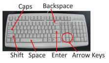
Fig 5.2.2 Basic parts of a Keyboard
