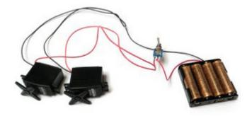
Figure 1.2.1 (C) 3 Parallel motor & Series Wiring
