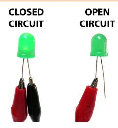
Figure 1.2.1 (B) Closed & Open Circuit
