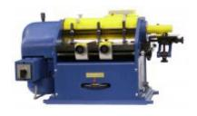
Fig.2.1.3.(K) Coil winding machine
