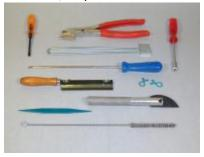
Fig.2.1.3.(J) Coil winding tools
