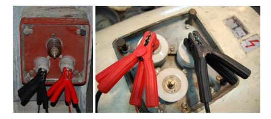
Figure 2 - Connection for measuring the stator winding resistance of induction motor
